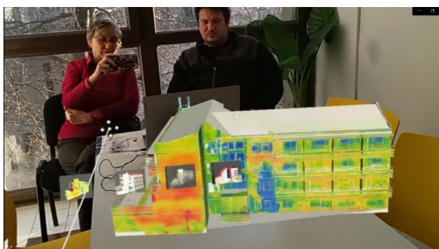
Fig.6 Hologram of CAD model, textured with thermal scans of the existing condition
