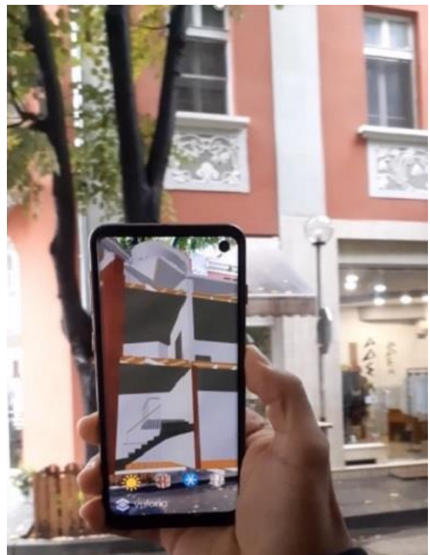
Fig.11 Mobile AR of a section of the BIM model of the building (virtually removed façade)
