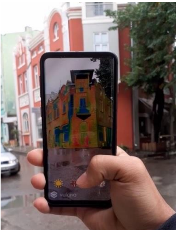
Fig.9 Mobile AR of the BIM model, textured by the 2D thermal scans from the thermal surveys
