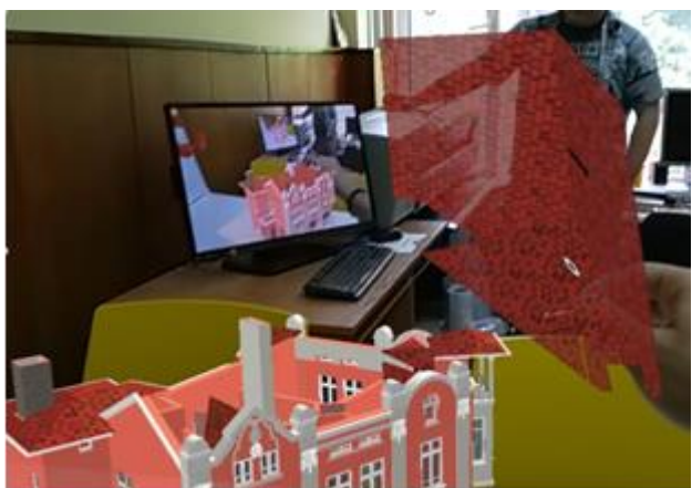
Fig.22 View from Microsoft HoloLens on a MR hologram in the moment of opening the roof and the parallel monitoring on a desktop
