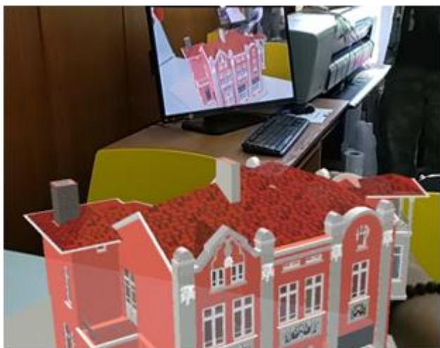
Fig.21 View from Microsoft HoloLens 2 on a MR hologram of a scaled BIM model, and the parallel monitoring on a desktop
