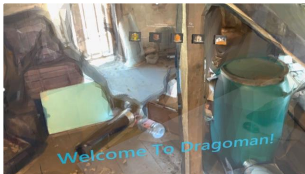
Fig.27 View of a photogrammetric model in scale 1:1 by Microsoft HoloLens 2
