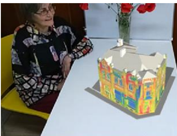
Fig.20 MR hologram of a scaled BIM model, textured with the 2D thermal scans from a survey with a thermo-visional FLIR camera
