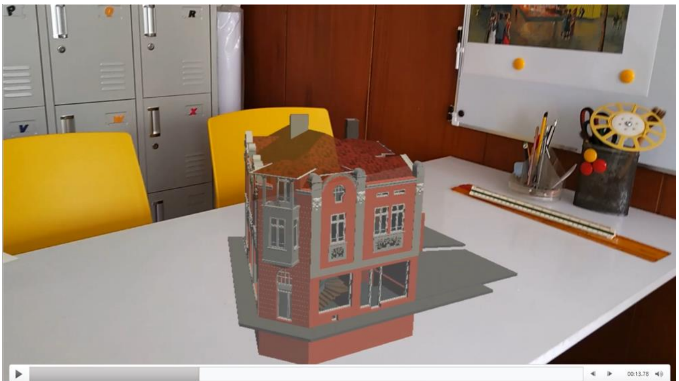
Fig. 2. Videorecording of the view from Microsoft Hololens-2 on the hologram of the BIM
